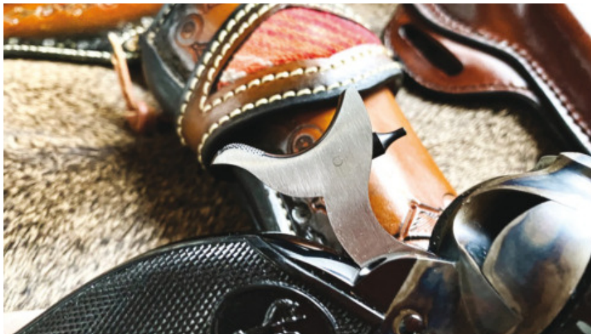
Colt firing pins are slightly tapered and have a square face. You'll see a great deal of variance in the hammers on import guns; many have a small safety lever and some even have Ruger-style transfer bars.
