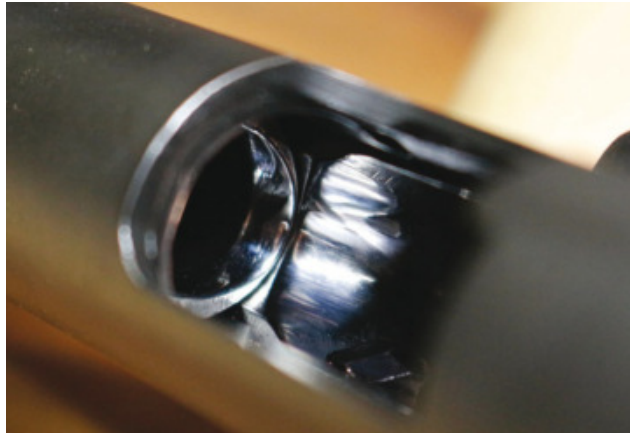
A rough feed ramp can pose a problem in some handguns, as certain bullet profiles may not feed. Get the feed ramp polished and you'll see an improvement immediately.
